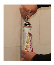
2. Rotate the gun or hand-adaptor on top of the foam cannister. Alsways keep the bottle upright when fastening the gun or adapter. Shake cannister at least 20 times in a vertical direction.
